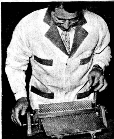
The brake is the principal sheet-metal tool. The unit shown here will handle sheet metal of 20-gauge thickness and up to 12 in. wide
